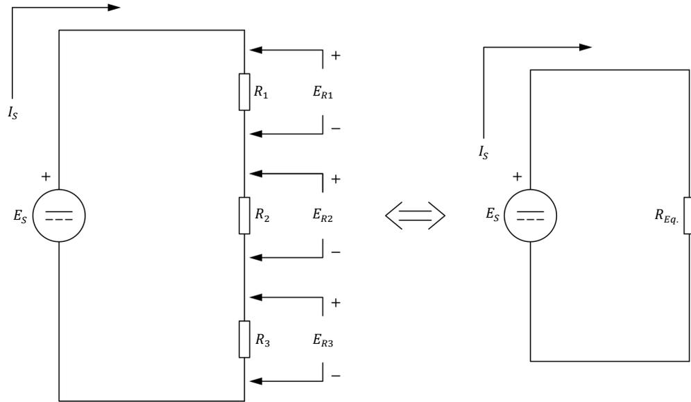
Figure 28. Simplification of a series circuit.
