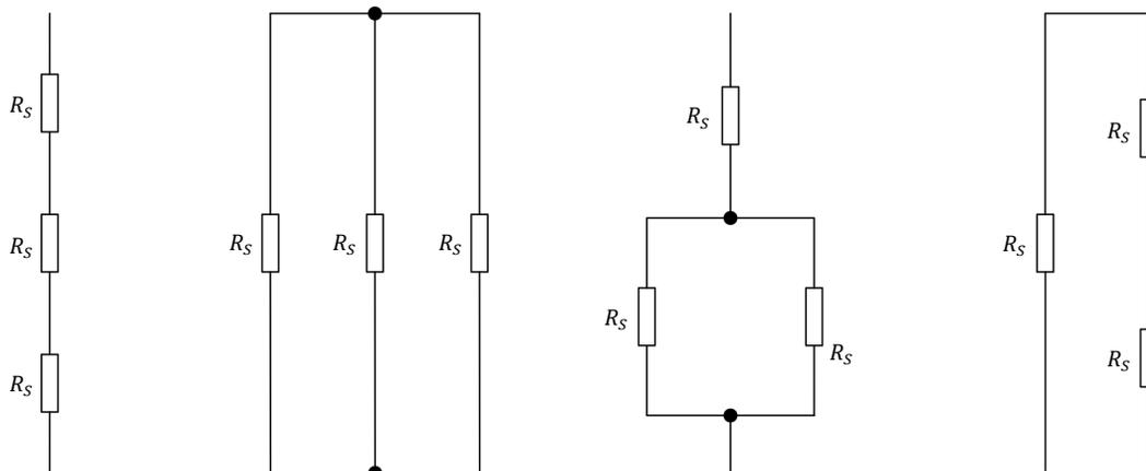
**Figure 17.** Any two or all three resistors of a section can be placed in parallel. Moreover, the resistor sections can be connected in series, in parallel or in series-parallel to obtain various resistor arrangements.
