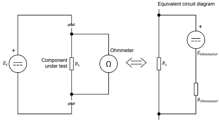
Figure 6. Measuring resistance with an ohmmeter.
