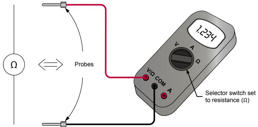
Figure 9. The multimeter is used as an ohmmeter.
